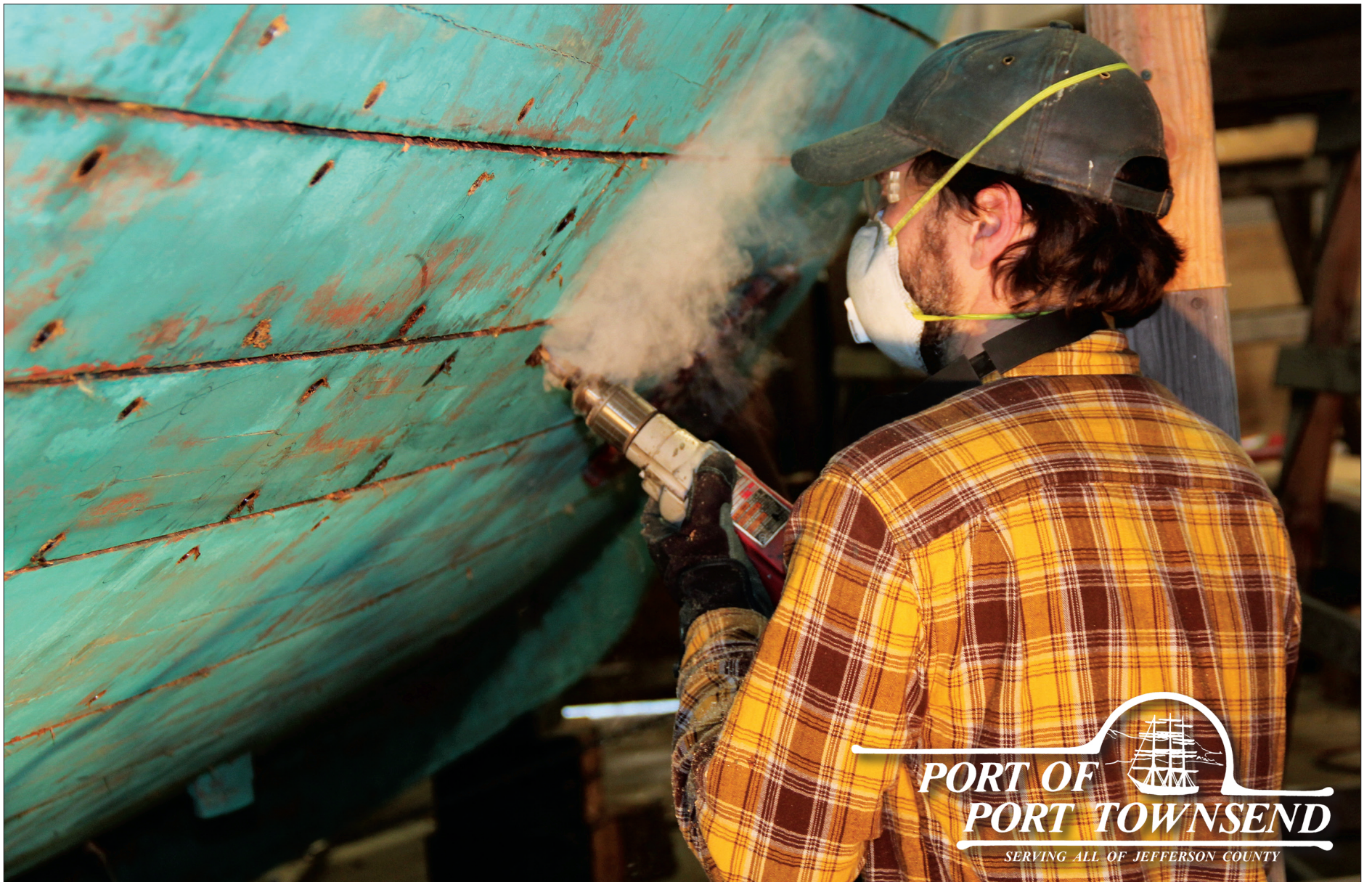
Gordon Kwiatkowski of Haven Boatworks looks through his drill bit's smoke and steam while refastening the hull of MV Carmelita.
